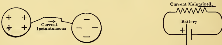
FIG. 10.—Indicating a difference between electro-motive force and potential difference. The two charged balls show no tendency to keep the current flowing after the discharge has passed, but the battery, by virtue of internal chemical action, will maintain its current for a long time.
